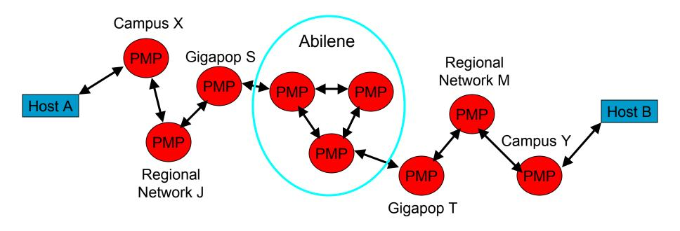
Regular tests are performed between adjacent PMP and stored in a Data Repository. This information is used by the End-User tool to reduce the number or active tests needed.
