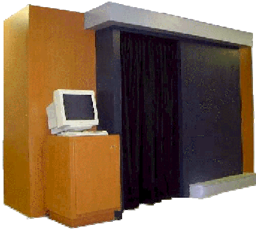
Fig. 4. Digital Body Measurement System with Enclosure
