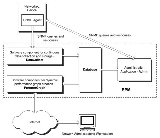
Figure 2. Structure of the network management application
