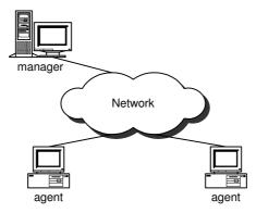
Figure 1. Generic model of a centralized network management system
