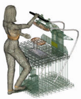
Fig. 6. Perspective Wireframe presentation of a simulation model of a worker at a workplace
