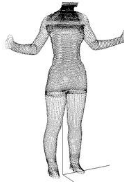
Fig. 5. 3D cloud of coordinate points of a virtual model of the actor scanned
