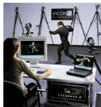
Fig. 8. Motion capture system Vicon with a passive reflex markers and high-resolution camcorders
